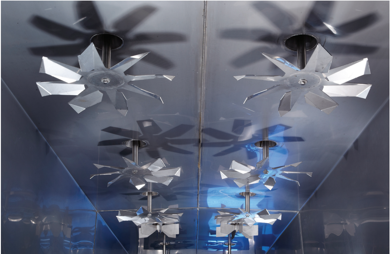
Gas-movement fans in a liquid nitrogen tunnel freezer facilitate heat transfer within the tunnel during chilling and freezing.
