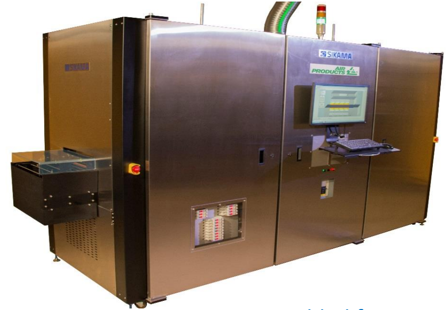
UP1200 EA-enabled furnace
