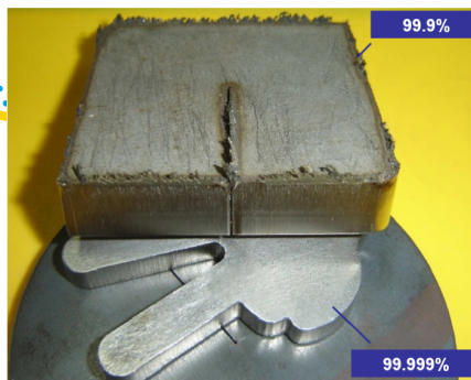
Figure 1: Comparison of identical metals cut with 99.9% and 99.999% pure nitrogen
