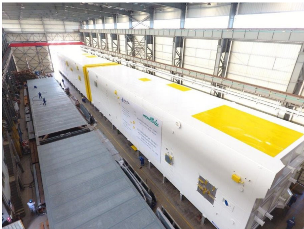
Figure 5. Cold boxes being manufactured at Air Products' Caojing manufacturing facility in Shanghai, China.
