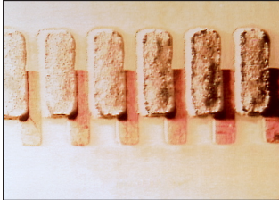
Figure 1: Air Versus Nitrogen Reflow
