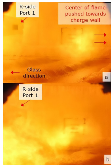
Figure 5: Right side oxy-fuel boost burners with opposed (left) side air-fuel burner firing. Figure 5a shows the HR_x burner that is not optimized, where the flame can be periodically pushed in the direction of the furnace charge end wall. Figure 5b shows the HR_x burner with synchronized boosting where the flame properties were optimized and were automatically tuned to increase momentum and stability and minimize the effects of localized turbulence
