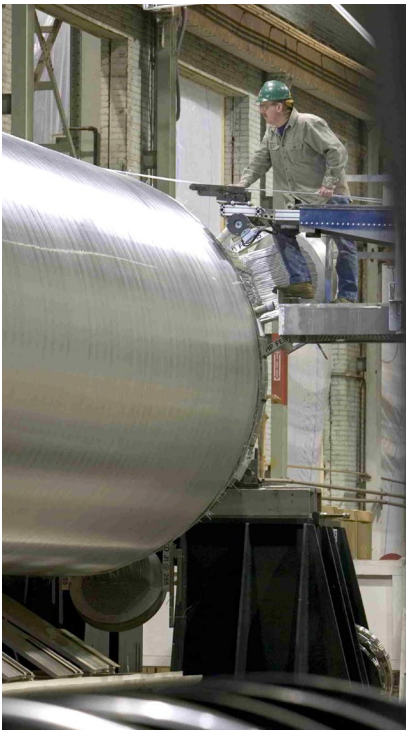
LNG heat exchanger bundle winding process.
